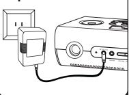
Attach AC adaptor cable to DC jack on back of the ZN90 and plug the other end into a wall socket.
